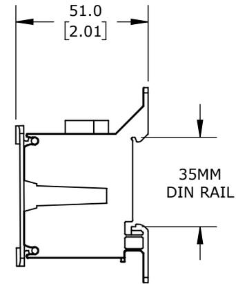
FINGER-SAFE, 115A, 3-POLE, LINE SIDE: 1 OPENING ACCEPTS 2 AWG TO 18 AWG, LOAD SIDE: 1 OPENING ACCEPTS 6 AWG TO 10 AWG & 6 OPENINGS ACCEPT 6 AWG TO 14 AWG, DIN RAIL OR PANEL MOUNT, UL 1059 RECOGNIZED.
