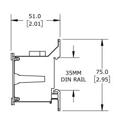
FINGER-SAFE, 115A, 1-POLE, LINE SIDE: 1 OPENING ACCEPTS 2 AWG TO 18 AWG, LOAD SIDE: 1 OPENING ACCEPTS 6 AWG TO 10 AWG & 6 OPENINGS ACCEPT 6 AWG TO 14 AWG, DIN RAIL OR PANEL MOUNT, UL 1059 RECOGNIZED.
