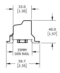
FINGER-SAFE, 85A, 1-POLE, LINE SIDE: 3 OPENINGS ACCEPT 6 AWG TO 16 AWG, LOAD SIDE: 4 OPENINGS ACCEPT 8 AWG TO 16 AWG, DIN RAIL OR PANEL MOUNT, UL 1059 RECOGNIZED.
