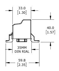
FINGER-SAFE, 85A, 1-POLE, LINE SIDE: 3 OPENINGS ACCEPT 6 AWG TO 16 AWG, LOAD SIDE: 12 OPENINGS ACCEPT 8 AWG TO 16 AWG, DIN RAIL OR PANEL MOUNT, UL 1059 RECOGNIZED.
