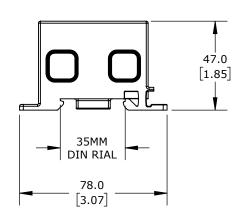
FINGER-SAFE, 130A, 1-POLE, LINE SIDE: 2 (SCREW) OPENINGS ACCEPT 1 AWG TO 8 AWG & 2 OPENINGS ACCEPT 6 AWG TO 16 AWG, LOAD SIDE: 12 OPENINGS ACCEPT 8 AWG TO 16 AWG, DIN RAIL OR PANEL MOUNT, UL 1059 RECOGNIZED.
