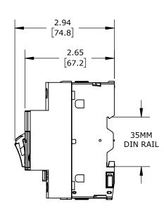
PUSHBUTTON, 25A, THERMAL OVERLOAD, 20-25 ADJUSTABLE, 327A INSTANTANEOUS TRIP RATING, 45mm FRAME.
