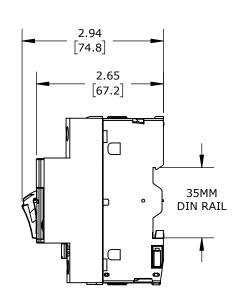
PUSHBUTTON, 18A, THERMAL OVERLOAD, 13-18 ADJUSTABLE, 223A INSTANTANEOUS TRIP RATING, 45mm FRAME.
