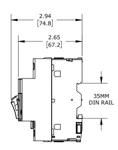
PUSHBUTTON, 14A, THERMAL OVERLOAD, 9-14 ADJUSTABLE, 170A INSTANTANEOUS TRIP RATING, 45mm FRAME.
