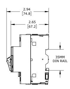
PUSHBUTTON, 6.3A, THERMAL OVERLOAD, 4-6.3 ADJUSTABLE, 78A INSTANTANEOUS TRIP RATING, 45mm FRAME.
