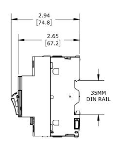
PUSHBUTTON, 4A, THERMAL OVERLOAD, 2.5-4 ADJUSTABLE, 51A INSTANTANEOUS TRIP RATING, 45mm FRAME.
