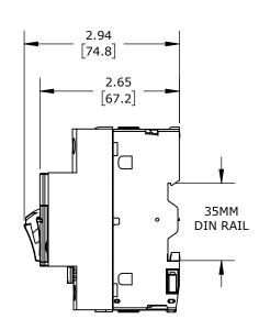
PUSHBUTTON, 0.63A, THERMAL OVERLOAD, 0.40-0.63 ADJUSTABLE, 8A INSTANTANEOUS TRIP RATING, 45mm FRAME.
