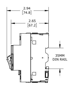
PUSHBUTTON, 0.4A, THERMAL OVERLOAD, 0.25-0.40 ADJUSTABLE, 5A INSTANTANEOUS TRIP RATING, 45mm FRAME.
