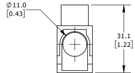
115A, 1000 VAC/VDC, 1 OPENINGS, 2 TO 14 AWG COPPER ONLY. PACKAGE OF 10. FOR USE WITH GLADIATOR GMCBU SERIES UL489 BUSBARS.
