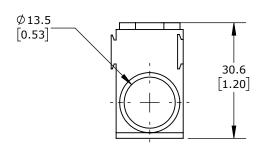
115A, 1000 VAC/VDC, 1 OPENINGS, 1 TO 14 AWG COPPER ONLY. PACKAGE OF 8. FOR USE WITH GLADIATOR GMCBU SERIES UL489 BUSBARS
