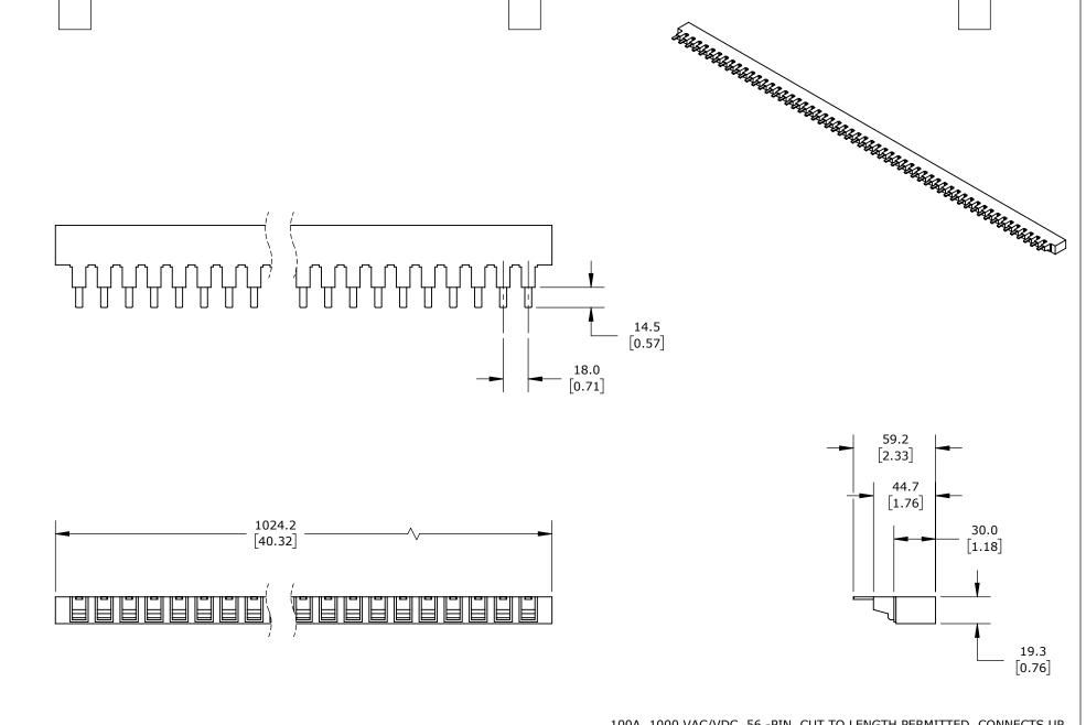
100A, 1000 VAC/VDC, 56 -PIN, CUT TO LENGTH PERMITTED, CONNECTS UP TO (28) 2-POLE GLADIATOR GMCBU SERIES MINIATURE CIRCUIT BREAKERS WITHOUT AUXILIARY COMPONENTS. (2) ENDCAPS INCLUDED.
