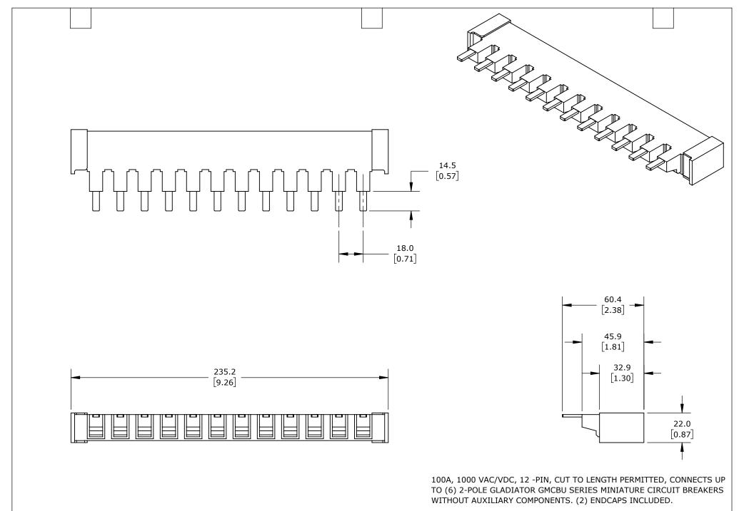
AutomationDirect.com **GLADIATOR BUSBAR** GMCBU-BB2P-12-100C 1-800-633-0405 METRIC UNITS USED UNLESS OTHERWISE 3rd PART DIMENSIONS MAY DIFFER SLIGHTLY mm LATEST VERSION NOT TO SHEET 1 OF 1 [inch] ANGLE FOR PART DESIGN SCALE DUE TO MANUFACTURER'S VARIANCES SPECIFIED UNITS ARE: 7/23/2024
