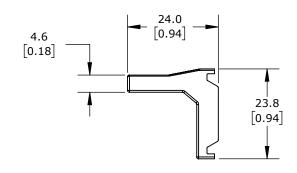
PACKAGE OF 10. FOR USE WITH UP TO (5) UNUSED PINS ON GLADIATOR GMCB SERIES BUSBARS.
