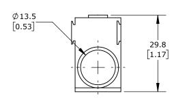
115A, 1000 VAC/VDC, 1 OPENINGS, 1 TO 14 AWG COPPER ONLY. PACKAGE OF 10. FOR USE WITH GLADIATOR GMCB SERIES UL1077 BUSBARS.
