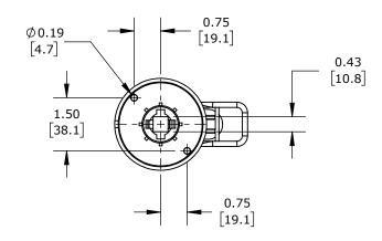
PISTOL, BLACK, EXTERNAL FRONT MOUNT, 2-POSITION, LOCKABLE IN OFF ONLY, DEFEATABLE, NEMA 1/12. FOR USE WITH AUTOMATIONDIRECT (EATON) 100A FRAME MCCBS. 12IN SHAFT AND OPERATOR INCLUDED.
