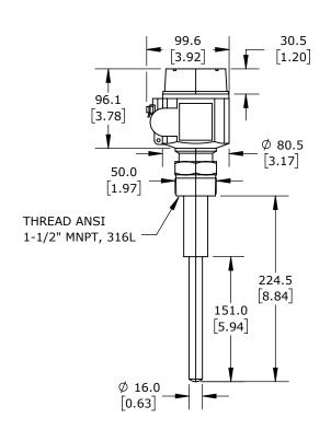
ENDRESS+HAUSER SOLIPHANT VIBRATION ROD BULK SOLIDS LEVEL SWITCH, ALUMINUM HOUSING, 8.86IN INSERTION LENGTH, 316L STAINLESS STEEL WETTED PARTS, 1-1/2IN MALE NPT PROCESS CONNECTION, SWITCH PNP, 3-WIRE, N.O./N.C. SELECTABLE, SCREW TERMINALS, HAZARDOUS LOCATION RATED
