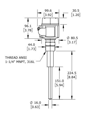
ENDRESS+HAUSER SOLIPHANT VIBRATION ROD BULK SOLIDS LEVEL SWITCH, ALUMINUM HOUSING, 8.86IN INSERTION LENGTH, 316L STAINLESS STEEL WETTED PARTS, 1-1/4IN MALE NPT PROCESS CONNECTION, DPDT RELAY, SCREW TERMINALS, HAZARDOUS LOCATION RATED
