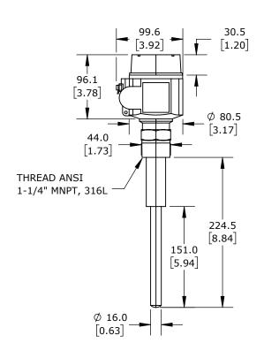
ENDRESS+HAUSER SOLIPHANT VIBRATION ROD BULK SOLIDS LEVEL SWITCH, ALUMINUM HOUSING, 8.86IN INSERTION LENGTH, 316L STAINLESS STEEL WETTED PARTS, 1-1/4IN MALE NPT PROCESS CONNECTION, SWITCH PNP, 3-WIRE, N.O./N.C. SELECTABLE, SCREW TERMINALS, HAZARDOUS LOCATION RATED
