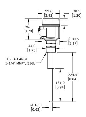
ENDRESS+HAUSER SOLIPHANT VIBRATION ROD BULK SOLIDS LEVEL SWITCH, ALUMINUM HOUSING, 8.86IN INSERTION LENGTH, 316L STAINLESS STEEL WETTED PARTS, 1-1/4IN MALE NPT PROCESS CONNECTION, DPDT RELAY, SCREW TERMINALS
