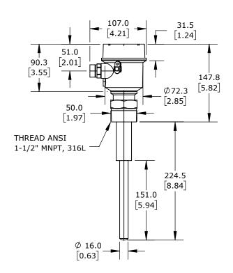
ENDRESS+HAUSER SOLIPHANT VIBRATION ROD BULK SOLIDS LEVEL SWITCH, POLYESTER HOUSING, 8.86IN INSERTION LENGTH, 316L STAINLESS STEEL WETTED PARTS, 1-1/2IN MALE NPT PROCESS CONNECTION, DPDT RELAY, SCREW TERMINALS
