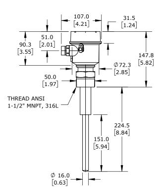
ENDRESS+HAUSER SOLIPHANT VIBRATION ROD BULK SOLIDS LEVEL SWITCH, POLYESTER HOUSING, 8.86IN INSERTION LENGTH, 316L STAINLESS STEEL WETTED PARTS, 1-1/2IN MALE NPT PROCESS CONNECTION, SWITCH PNP, 3-WIRE, N.O./N.C. SELECTABLE, SCREW TERMINALS
