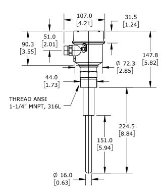
ENDRESS+HAUSER SOLIPHANT VIBRATION ROD BULK SOLIDS LEVEL SWITCH, POLYESTER HOUSING, 8.86IN INSERTION LENGTH, 316L STAINLESS STEEL WETTED PARTS, 1-1/4IN MALE NPT PROCESS CONNECTION, DPDT RELAY, SCREW TERMINALS
