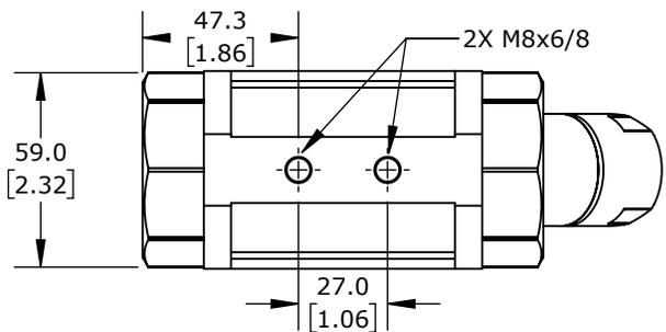
PROSENSE LIQUID DIGITAL FLOW SENSOR, SPRING-SUPPORTED PISTON, 1-1/2IN FEMALE NPT PROCESS CONNECTION, 0 TO 50 GPM, 14 TO 212 DEG F, OUTPUT: SWITCH OR FREQUENCY, OUTPUT 2: SWITCH OR CURRENT, 18 TO 30 VDC OPERATING VOLTAGE
