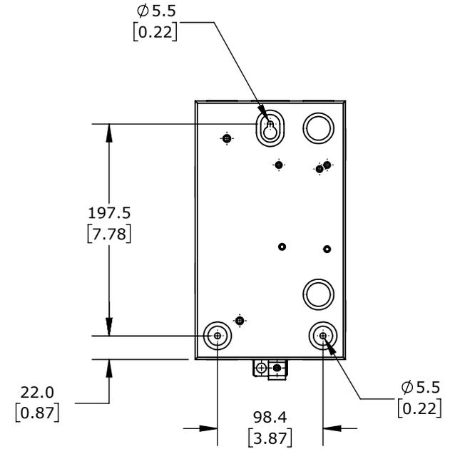
9A, 2-POLE, 120 VAC (50/60Hz) COIL VOLTAGE, THERMAL
