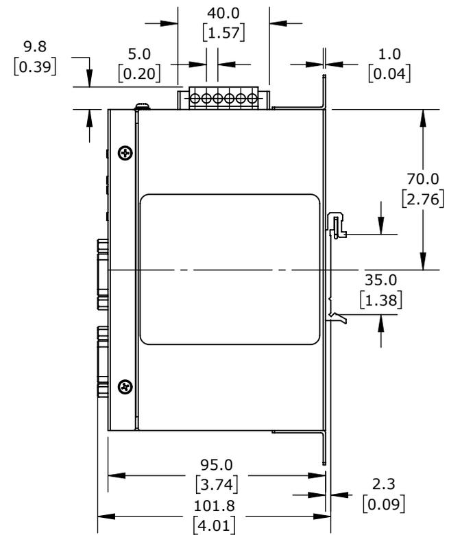
ADVANTECH MODBUS GATEWAY, SERIAL MASTER/SLAVE AND ETHERNET CLIENT/SERVER, (2) ETHERNET 10/100BASE-T (RJ45) AND (2) RS-232/422/485 (9-PIN D-SUB MALE) PORT(S), (64) SIMULTANEOUS ETHERNET CONNECTIONS, (64) SERIAL DEVICE(S), 12-48 VDC REQUIRED
