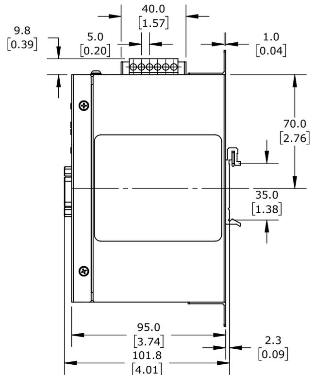
ADVANTECH MODBUS GATEWAY, SERIAL MASTER/SLAVE AND ETHERNET CLIENT/SERVER, (2) ETHERNET 10/100BASE-T (RJ45) AND (1) RS-232/422/485 (9-PIN D-SUB MALE) PORT(S), (64) SIMULTANEOUS ETHERNET CONNECTIONS, (32) SERIAL DEVICE(S), 12-48 VDC REQUIRED
