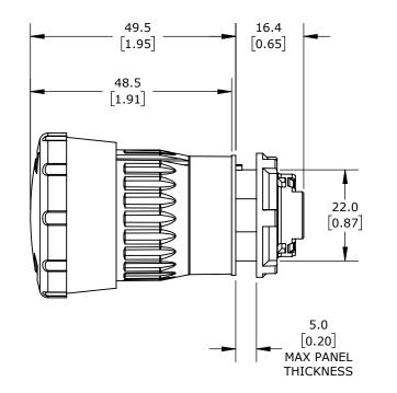
IP65, 22mm, TWIST-TO-RELEASE, OPERATOR ONLY, THERMOPLASTIC BASE, THERMOPLASTIC BEZEL, OPERATOR: RED, MUSHROOM, 40mm, MUSHROOM, PLASTIC, OPERATOR TEXT "ARROW". REQUIRES ECX4029-2 MOUNTING FLANGE AND ECX10X0N-2 CONTACT BLOCK.
