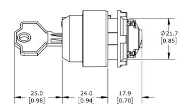
IP65, 22mm, 2-POSITION, MAINTAINED, KEY REMOVABLE LEFT POSITION, OPERATOR ONLY, THERMOPLASTIC BASE, THERMOPLASTIC BEZEL, OPERATOR: BLACK, KEY-OPERATED, 30mm, ROUND. REQUIRES ECX4029-2 MOUNTING FLANGE AND ECX10X0N-2 CONTACT BLOCK.
