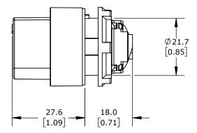
IP65, 22mm, 3-POSITION, MAINTAINED, OPERATOR ONLY, THERMOPLASTIC BASE, THERMOPLASTIC BEZEL, OPERATOR: BLACK, LEVER, 30mm, ROUND. REQUIRES ECX4029-2 MOUNTING FLANGE AND ECX10X0N-2 CONTACT BLOCK.
