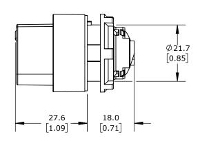
IP65, 22mm, 2-POSITION, MAINTAINED, OPERATOR ONLY, THERMOPLASTIC BASE, THERMOPLASTIC BEZEL, OPERATOR: BLACK, KNOB, 30mm, ROUND. REQUIRES ECX4029-2 MOUNTING FLANGE AND ECX10X0N-2 CONTACT BLOCK
