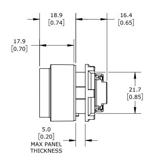
IP65, 22mm, MOMENTARY, OPERATOR ONLY, THERMOPLASTIC BASE, THERMOPLASTIC BEZEL, OPERATOR: RED, EXTENDED, 30mm, ROUND, PLASTIC. REQUIRES ECX4029-2 MOUNTING FLANGE AND ECX10X0N-2 CONTACT BLOCK.
