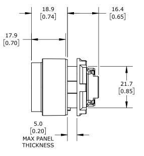
IP65, 22mm, MOMENTARY, OPERATOR ONLY, THERMOPLASTIC BASE, THERMOPLASTIC BEZEL, OPERATOR: RED, EXTENDED, 30mm, ROUND, PLASTIC, OPERATOR TEXT "(O)". REQUIRES ECX4029-2 MOUNTING FLANGE AND ECX10X0N-2 CONTACT BLOCK.
