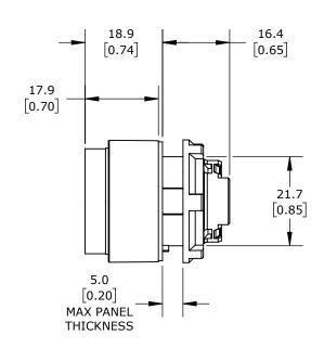
IP65, 22mm, MOMENTARY, OPERATOR ONLY, THERMOPLASTIC BASE, THERMOPLASTIC BEZEL, OPERATOR: BLACK, EXTENDED, 30mm, ROUND, PLASTIC, OPERATOR TEXT "STOP". REQUIRES ECX4029-2 MOUNTING FLANGE AND ECX10X0N-2 CONTACT BLOCK.
