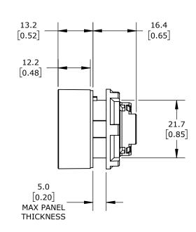
IP65, 22mm, MOMENTARY, OPERATOR ONLY, THERMOPLASTIC BASE, THERMOPLASTIC BEZEL, OPERATOR: BLACK, FLUSH, 30mm, ROUND, PLASTIC, OPERATOR TEXT "DOWN ARROW". REQUIRES ECX4029-2 MOUNTING FLANGE AND ECX10X0N-2 CONTACT BLOCK.
