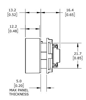
IP65, 22mm, MOMENTARY, OPERATOR ONLY, THERMOPLASTIC BASE, THERMOPLASTIC BEZEL, OPERATOR: WHITE, FLUSH, 30mm, ROUND, PLASTIC, OPERATOR TEXT "UP ARROW". REQUIRES ECX4029-2 MOUNTING FLANGE AND ECX10X0N-2 CONTACT BLOCK.
