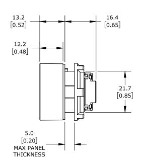
IP65, 22mm, MOMENTARY, OPERATOR ONLY, THERMOPLASTIC BASE, THERMOPLASTIC BEZEL, OPERATOR: GREEN, FLUSH, 30mm, ROUND, PLASTIC, OPERATOR TEXT "(I)". REQUIRES ECX4029-2 MOUNTING FLANGE AND ECX10X0N-2 CONTACT BLOCK.
