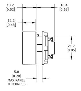
IP65, 22mm, MOMENTARY, OPERATOR ONLY, THERMOPLASTIC BASE, THERMOPLASTIC BEZEL, OPERATOR: RED, FLUSH, 30mm, ROUND, PLASTIC, OPERATOR TEXT "(O)". REQUIRES ECX4029-2 MOUNTING FLANGE AND ECX10X0N-2 CONTACT BLOCK.
