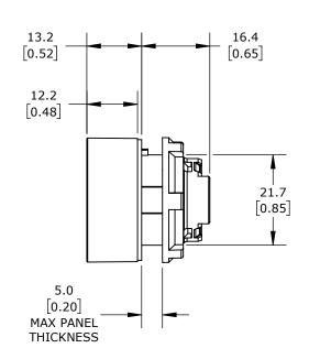
IP65, 22mm, MOMENTARY, OPERATOR ONLY, THERMOPLASTIC BASE, THERMOPLASTIC BEZEL, OPERATOR: WHITE, FLUSH, 30mm, ROUND, PLASTIC, OPERATOR TEXT "START". REQUIRES ECX4029-2 MOUNTING FLANGE AND ECX10X0N-2 CONTACT BLOCK.
