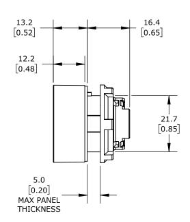
IP65, 22mm, MOMENTARY, OPERATOR ONLY, THERMOPLASTIC BASE, THERMOPLASTIC BEZEL, OPERATOR: BLUE, FLUSH, 30mm, ROUND, PLASTIC, OPERATOR TEXT "RESET". REQUIRES ECX4029-2 MOUNTING FLANGE AND ECX10X0N-2 CONTACT BLOCK.
