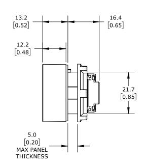
IP65, 22mm, MOMENTARY, OPERATOR ONLY, THERMOPLASTIC BASE, THERMOPLASTIC BEZEL, OPERATOR: GREEN, FLUSH, 30mm, ROUND, PLASTIC. REQUIRES ECX4029-2 MOUNTING FLANGE AND ECX10X0N-2 CONTACT BLOCK.
