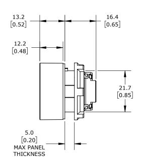
IP65, 22mm, MOMENTARY, OPERATOR ONLY, THERMOPLASTIC BASE, THERMOPLASTIC BEZEL, OPERATOR: RED, FLUSH, 30mm, ROUND, PLASTIC. REQUIRES ECX4029-2 MOUNTING FLANGE AND ECX10X0N-2 CONTACT BLOCK.
