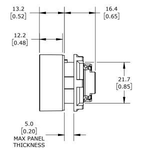
IP65, 22mm, MOMENTARY, OPERATOR ONLY, THERMOPLASTIC BASE, THERMOPLASTIC BEZEL, OPERATOR: BLACK, FLUSH, 30mm, ROUND, PLASTIC. REQUIRES ECX4029-2 MOUNTING FLANGE AND ECX10X0N-2 CONTACT BLOCK.
