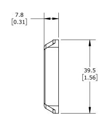
THERMOPLASTIC, BLACK. PACKAGE OF 2. FOR USE WITH COMEPI 22mm PUSHBUTTONS.
