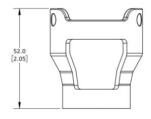
YELLOW. FOR USE WITH COMEPI 22mm PUSHBUTTONS. FOR EMERGENCY STOP APPLICATIONS.
