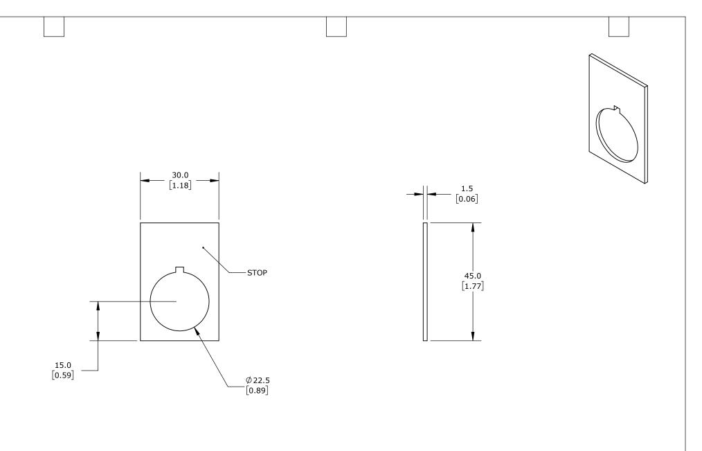
PLASTIC, RECTANGULAR, RED FIELD, RED BACKGROUND, WHITE ENGRAVED TEXT, LEGEND PLATE MARKING "STOP". FOR USE WITH 22mm PILOT DEVICES.
