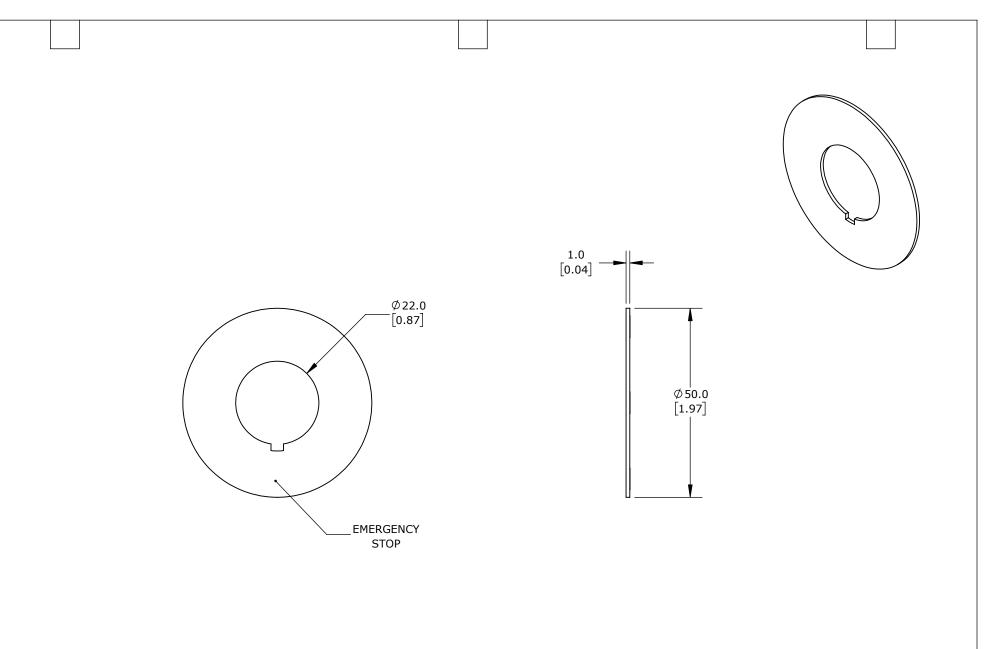
PLASTIC, ROUND, YELLOW FIELD, YELLOW BACKGROUND, BLACK ENGRAVED TEXT, LEGEND PLATE MARKING "EMERGENCY STOP". FOR USE WITH 22mm PILOT DEVICES.
